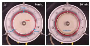
Fig. 1 (a) Experimental setup and (b) photographs taken at 0 and 30 minutes after the start of water infiltration showing the bentonite turning dark with saturation
